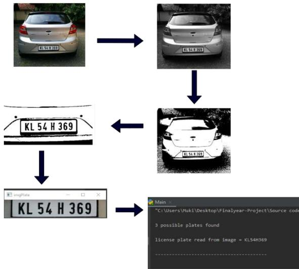
Fig -4: Steps for Detecting Number Plate
