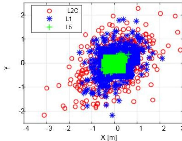
**Fig. 3** Position coordinate variation computed based on L1, L2 and L5 observations
