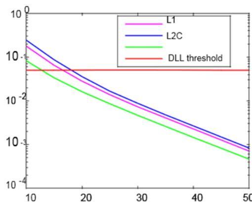
**Fig. 1** Comparison of 1-sigma code phase error variation with C/N0 in GPS L1, L2, and L5 signal code tracking loops
