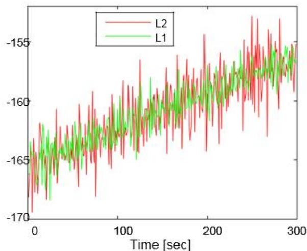
**Fig. 2** Comparison of GPS L1 and L2 code pseudorange rate
