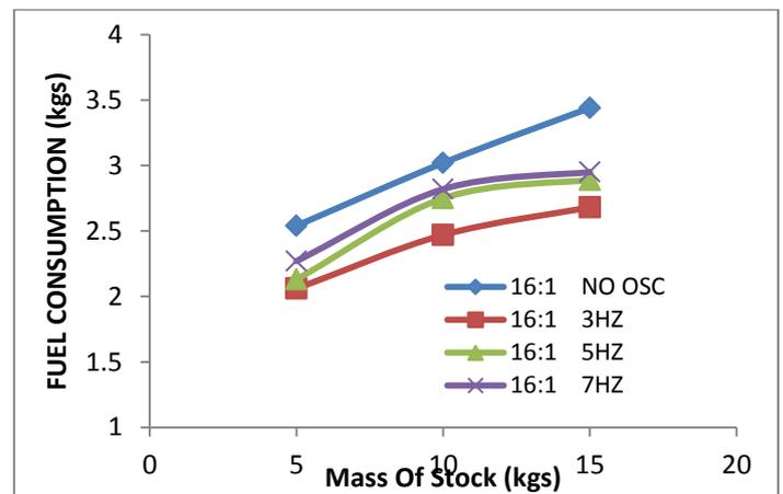
Figure 10 The Correlation between the load (MOS) and Fuel Consumption.
