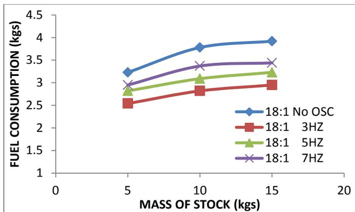
Figure 15 The Correlation between the load (MOS) and Fuel Consumption.
