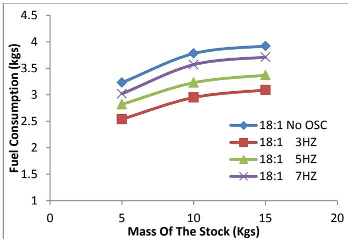
Figure 12 The Correlation between the load (MOS) and Fuel Consumption.
