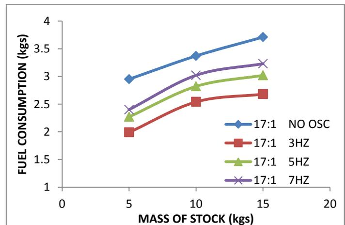
Figure 14 The Correlation between the load (MOS) and Fuel Consumption
