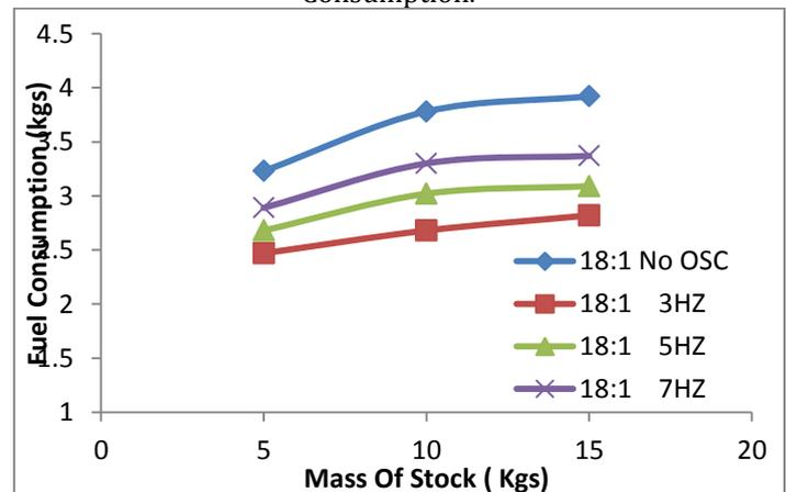
Figure 18 The Correlation between the load (MOS) and Fuel Consumption.
