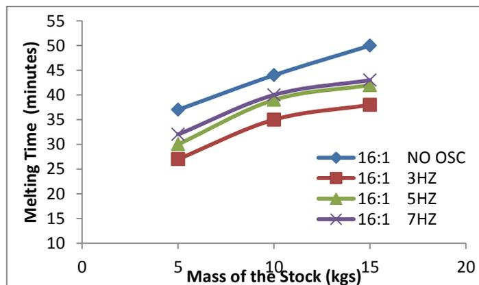
Figure 4 The plot between the load (MOS) and processing (melting) time.
