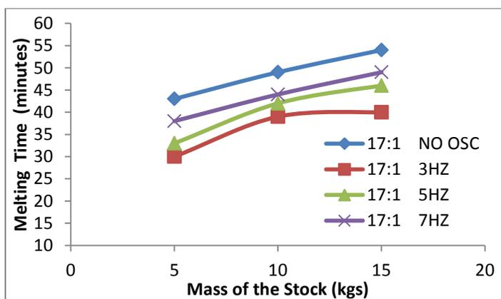
Figure 2 The plot between the load (MOS) and processing (melting) time
