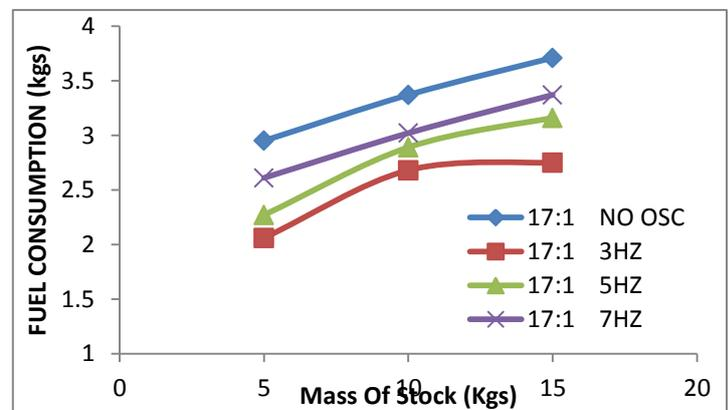
Figure 11 The Correlation between the load (MOS) and Fuel Consumption
