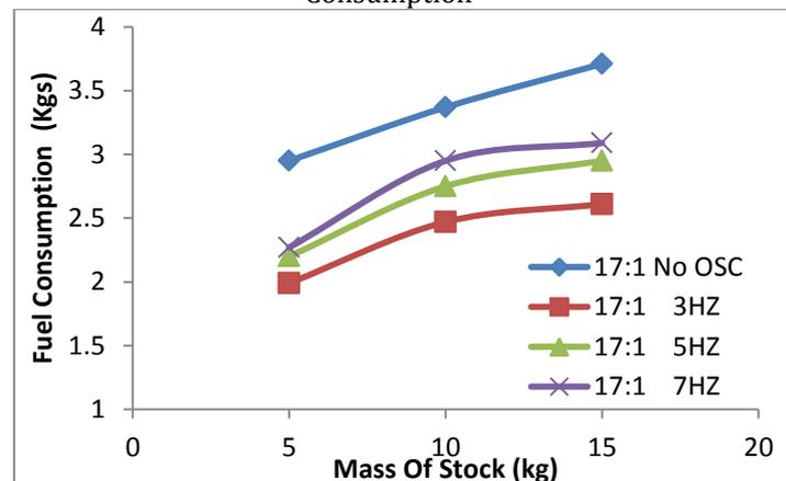
Figure 17 The Correlation between the load (MOS) and Fuel Consumption.
