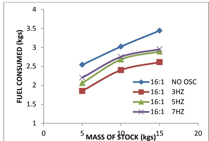
Figure 13 The Correlation between the load (MOS) and Fuel Consumption
