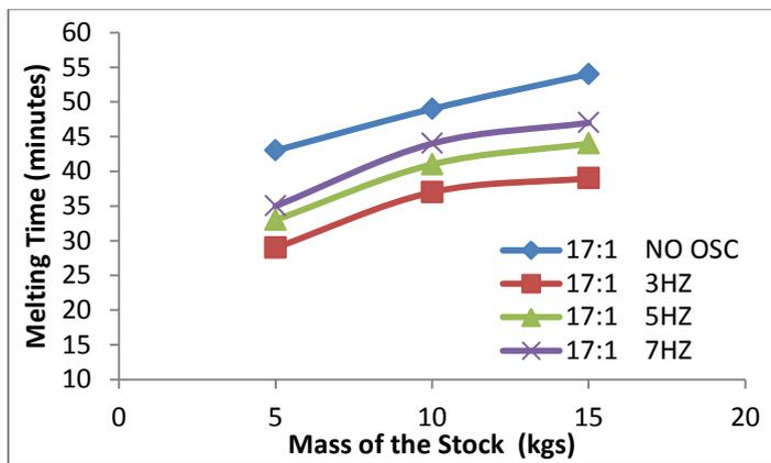
Figure 5 The plot between the load (MOS) and processing (melting) time.
