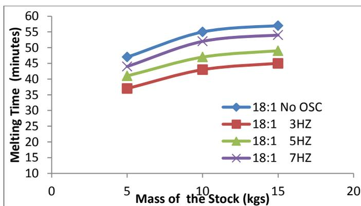
Figure 3 The plot between the load (MOS) and processing (Melting) time.
