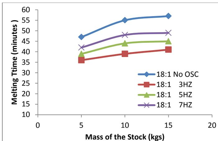
Figure 9 The plot between the mass of the stock and processing time.
