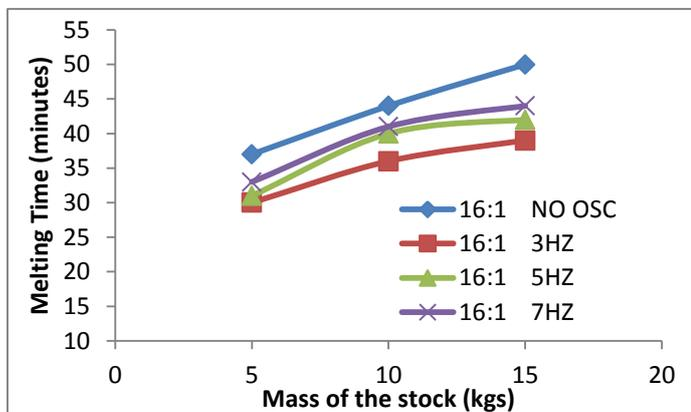
Figure 1 The plot between the load (MOS) and processing time
