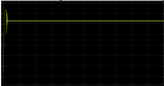
Fig 9 variation of PV voltage with time for G=800 w/m^2
