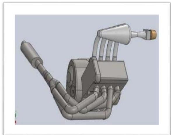
Fig 2: Assembled View of Manifold
