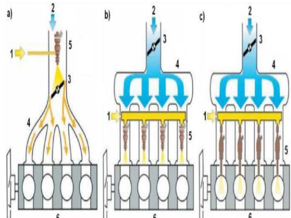
Fig 1: Systems of fuel injection
