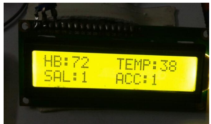
Fig. 12 LCD display showing values sensed by sensors
