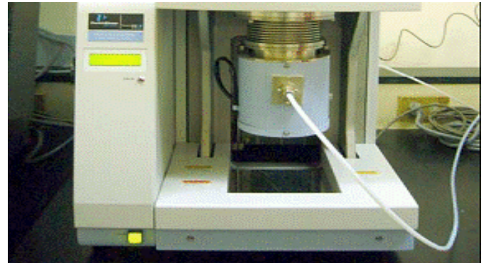
Fig. 4a. Loading of PETG specimen in DMA
