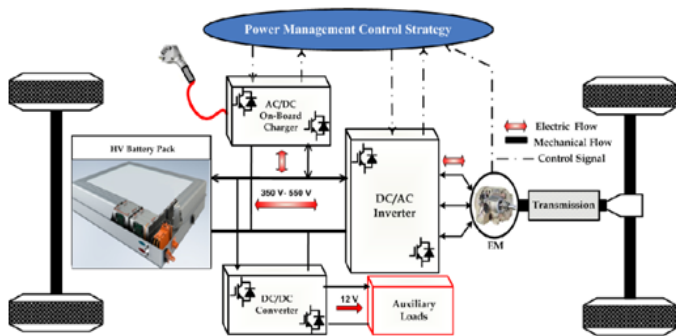
Figure 33: Power Conversion in Electric Vehicles [28]
