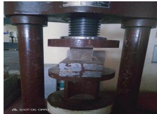
Fig 5: compression testing of cubes
