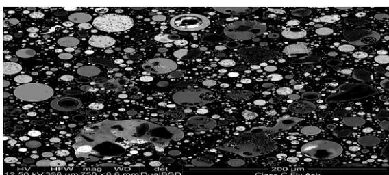
**Fig 1: SEM image of fly ash**
