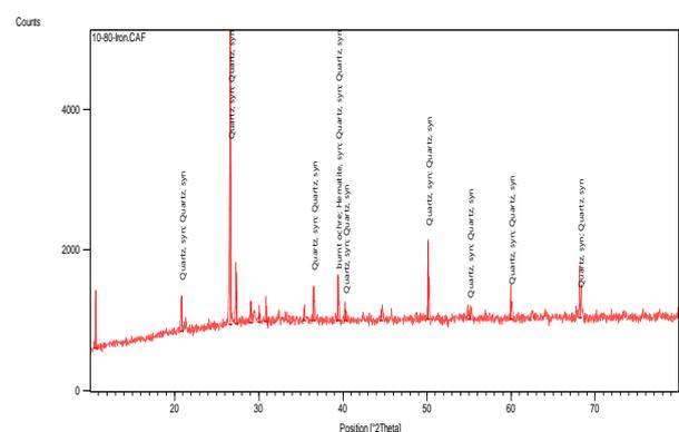
**Fig 3: X Ray diffraction pattern of Iron Ore Tailings**
