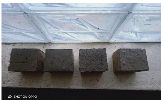
fig 4: 75mm cubes of different molarity
