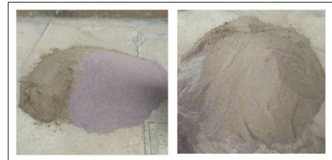
Fig-4: (Clay + Garnet sand) media preparation
