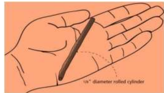
Figure 6: Rolled Cylinder for Plastic Limit test
