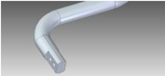
Figure 8. Punching process used to obtain holes for fixing screws.
