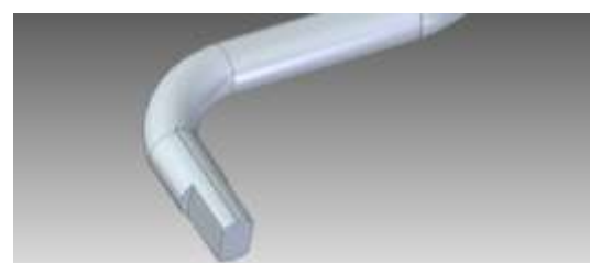
Figure 7. Stamping process used to obtain a flat surface for easy assembly.
