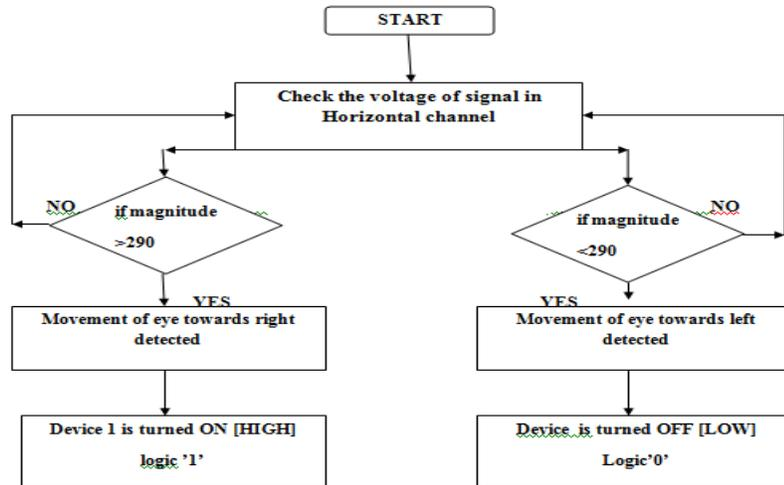
Fig. 7: Flowchart for detecting right-left eye movement
