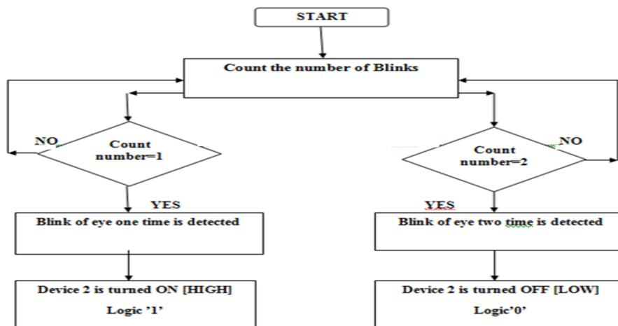
Fig. 6: Flowchart for blink detection
