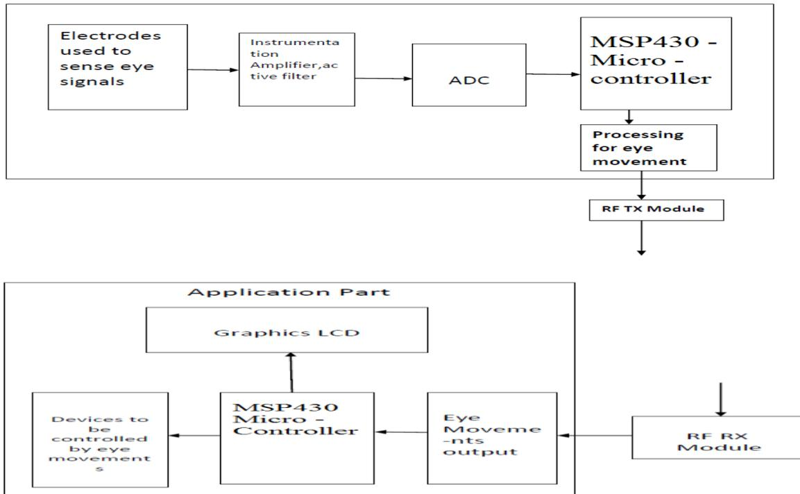
Fig. 3: EOG Block Diagram of the System
