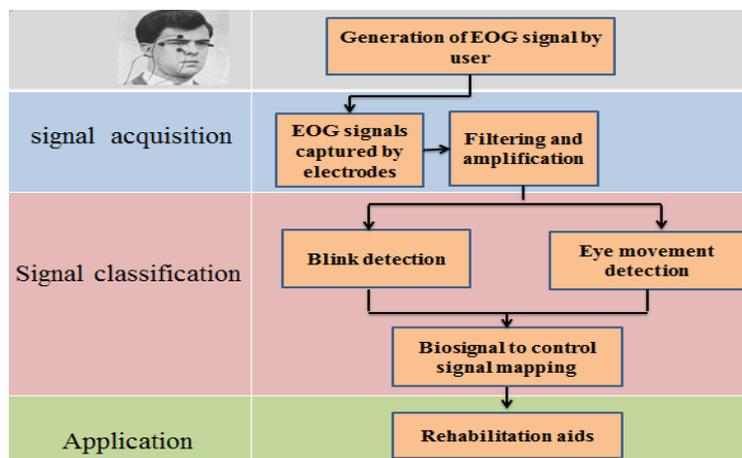
Fig. 4: Basic Block Diagram of EOG based HMI system
