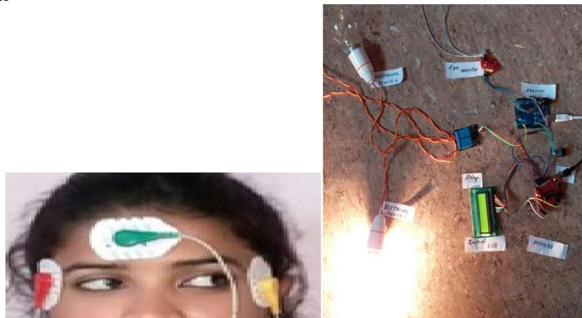
Fig. 8: Left eye movement was detected and device-1 is turned ON
