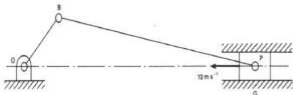
Fig -1: Slider Crank Mechanism
