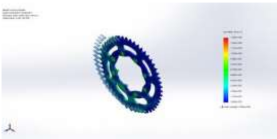
Fig - 45: Static analysis of sprocket
