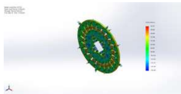
Fig - 42: Brake Disc thermal analysis
