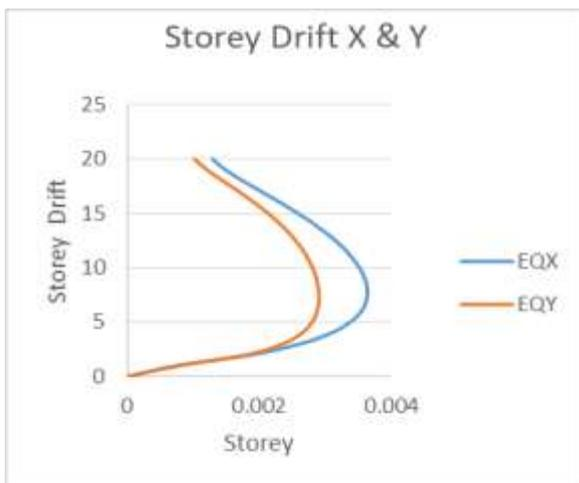
Fig 6.2: Storey drift in X and Y
