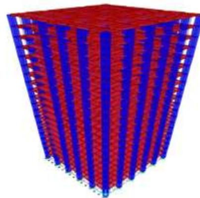
Fig 5.1 3D elevation view of 20 storey Flat slab building
