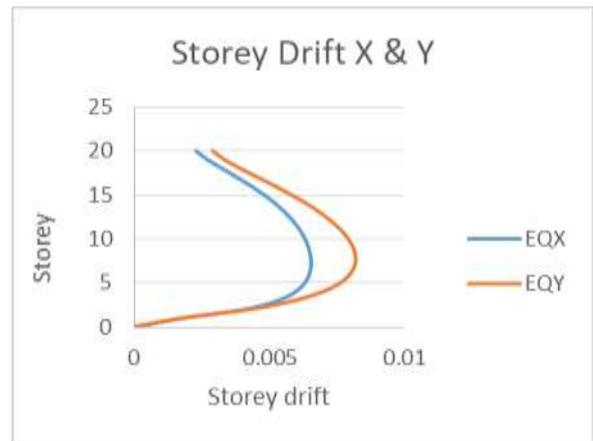
Fig 6.4: Storey drift in X and Y
