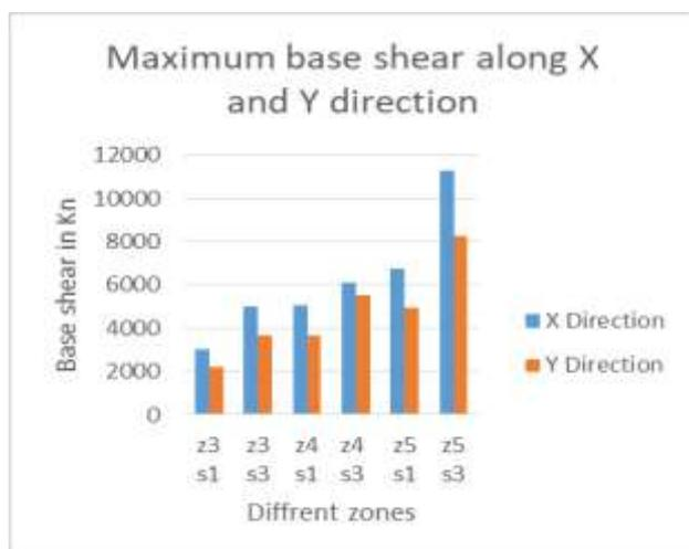
Fig 6.9: Base shear in X and Y direction
