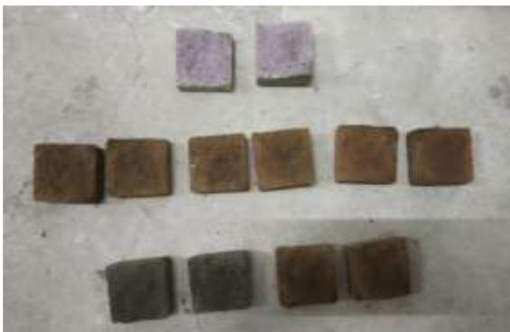
The conventional concrete block shows pink colour indications in the centre part which indicates non-carbonated part. The Ferrock blocks have no traces of pink indication which implies that the Ferrock has absorbed carbon dioxide for its hardening process and it is fully carbonated. The carbonation depths are displayed in Fig 3.a. & 3.b.
