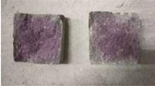
**Fig 3.b.** Carbonation depth of Ferrock Blocks
