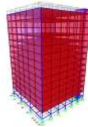
Fig -7: Plan regular frame with Soft storey at GF
