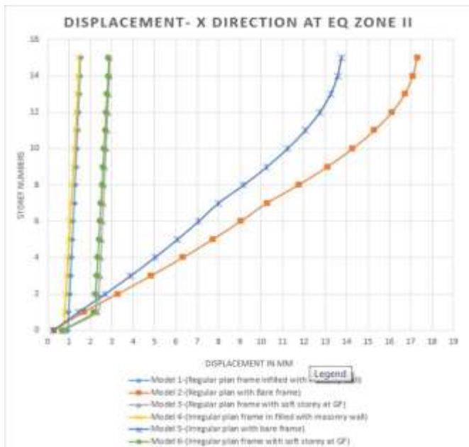
Fig -11: Displacement along X direction at zone II
