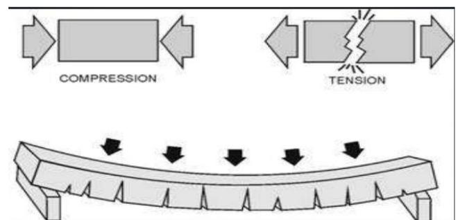
**COMPRESSION AND TENSION TEST**
