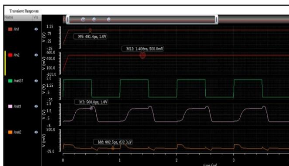
Fig. 4. Transient response of double tail comparator in 16t configuration
