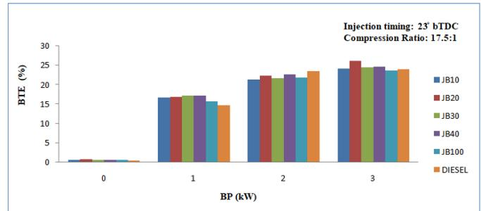
Fig.3.1 Variation of BTE with respect to brake Power
