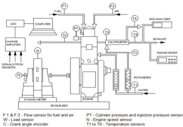
Fig.1. Schematic diagram of the Experimental Set up
