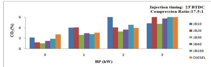
Fig.3.5 Variation of CO2 emissions with respect to brake Power
