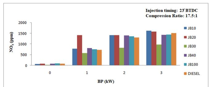
Fig.3.6 Variation of NOX emissions with respect to brake Power
