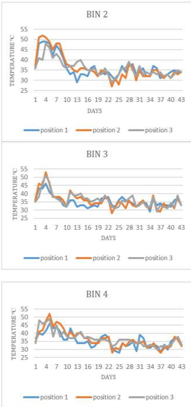
Fig.10 Temperature variations of Bin 1, Bin 2, Bin 3, Bin 4 for different vertical positions
