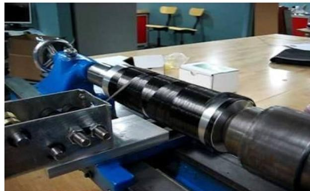
**Fig.3 filament winding Se-up**
