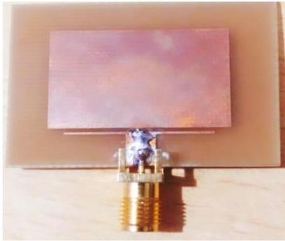
Fig 6:- Fabricated antenna
