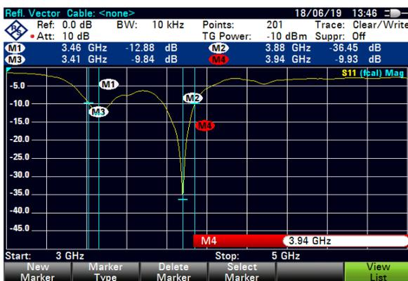
Fig 7:- S11 results on VNA of the proposed antenna
