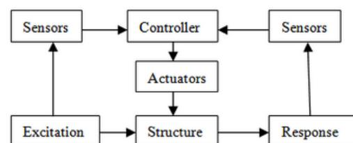
Fig. 2 Structure with Active Control System
