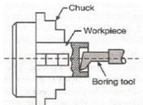
Fig. 1 Boring operation on a lathe
