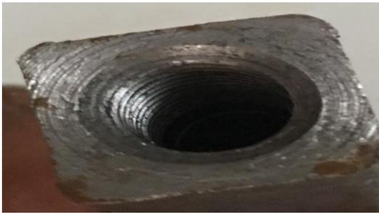
Fig.10 Hole at End for Oil (8mm Diameter)
