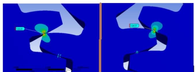
Figure- 6: Maximum Contact Stress Module 1 & 1.25
