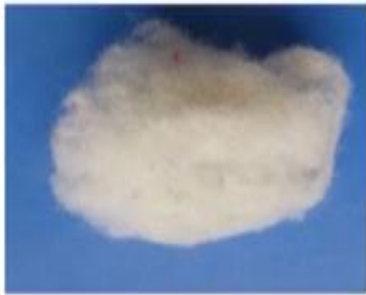
Cellulose acetate after the recycling process, ready to be used to produce other finished products.
