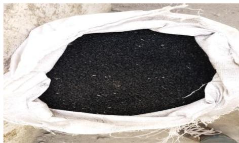
**Figure -1:** Actual photo of crumb rubber in size 2.36-4.75 mm
