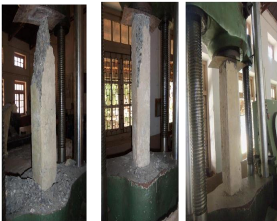
Figure 1: Failure Pattern of Unconfined Different Grades of Concrete Columns
