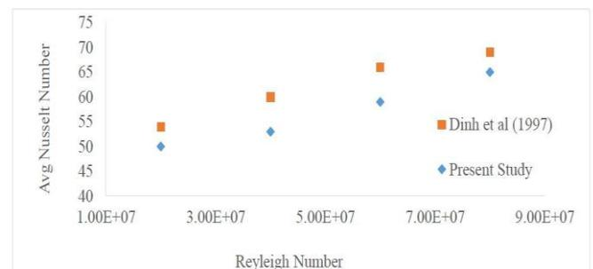
Fig 3. Variation of heat transfer coefficient with Rayleigh number
