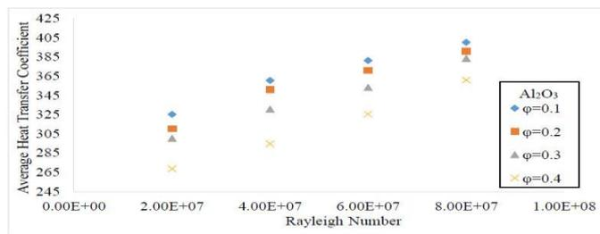
Fig. 4 Variation of average heat transfer coefficient with particle concentration of Al<sub>2</sub>O<sub>3</sub>
