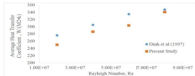
Fig 2 Variation of heat transfer coefficient with Rayleigh number
