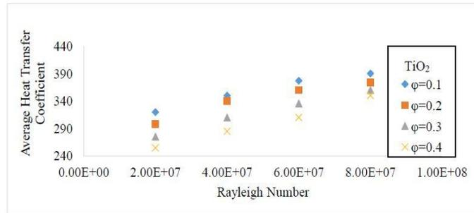
Fig 3 Variation of average heat transfer coefficient with particle concentration of TiO<sub>2</sub>
