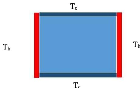
Fig 1 Flow configuration with horizontal walls are kept at  $T_c$  and vertical walls are kept at  $T_h$
