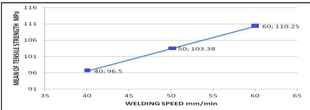
Fig 3.5: Variation of mean of tensile strength at different welding speeds
