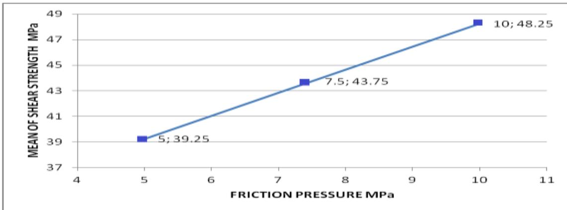
Fig 3.6: Variation of mean of shear strength at different friction pressures
