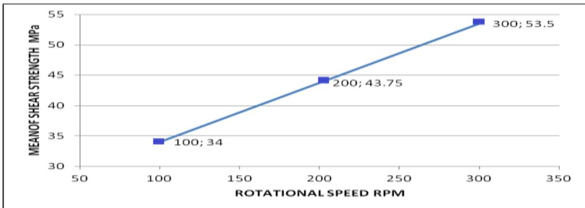
Fig 3.7: Variation of mean of shear strength at different rotational speeds
