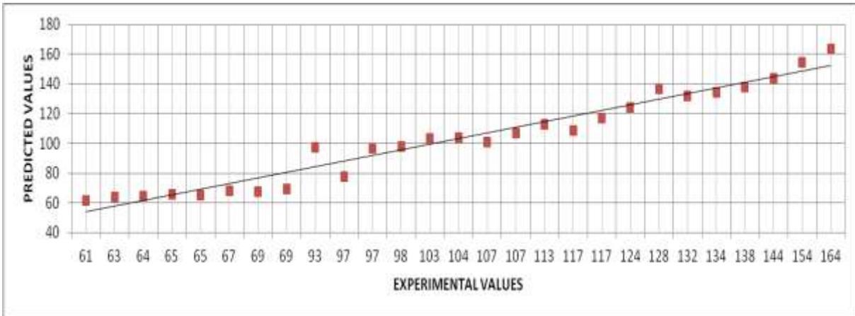
Fig. 4.1. Depicts the variation of predicted and experimental values of tensile strength of the deposit by using FFNN
