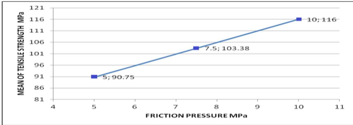
Fig 3.3: Variation of mean of tensile strength at different friction pressures
