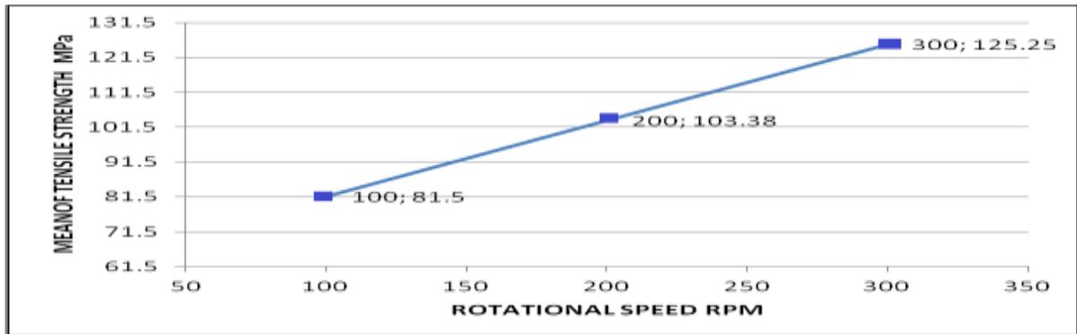
Fig 3.4: Variation of mean of tensile strength at different rotational speeds
