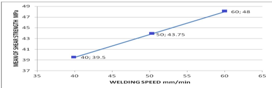
Fig 3.8: Variation of mean of shear strength with welding speeds
