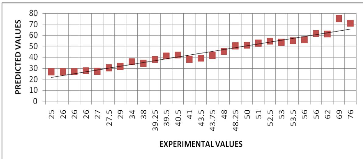
Fig 4.2: Predicted Vs Experimental Values for Shear Strength
