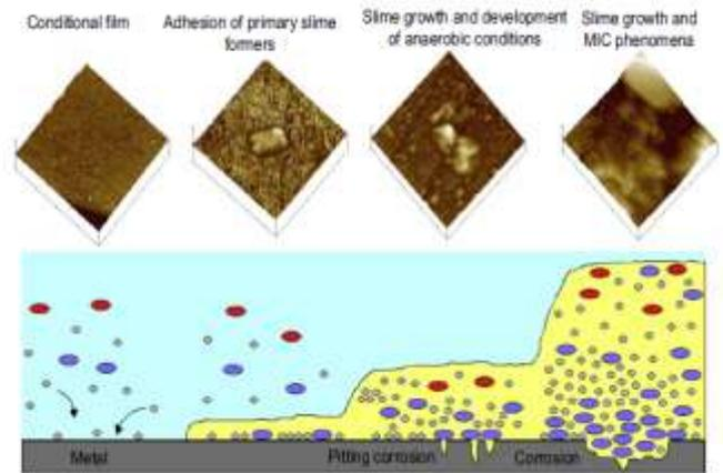
**Figure 3:** Biofilm formation step by Step
