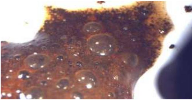
**Figure 2:** Azide spot test showing high rate of nitrogen bubble evolution, indicating positive indication of SRB
