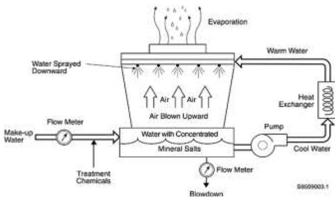
Figure 1: Function of cooling tower
