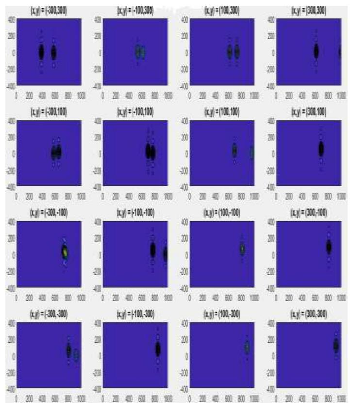
Fig-2: Collection of Range-Doppler maps for receiver array with two simulated targets
