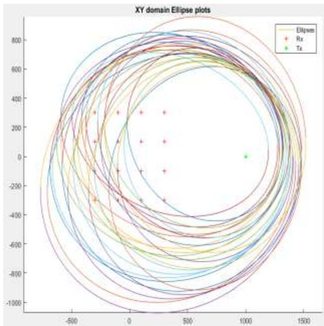
**Fig-3:** Spatial domain plot of all receivers, transmitters, and Range-Doppler map transformed ellipses
