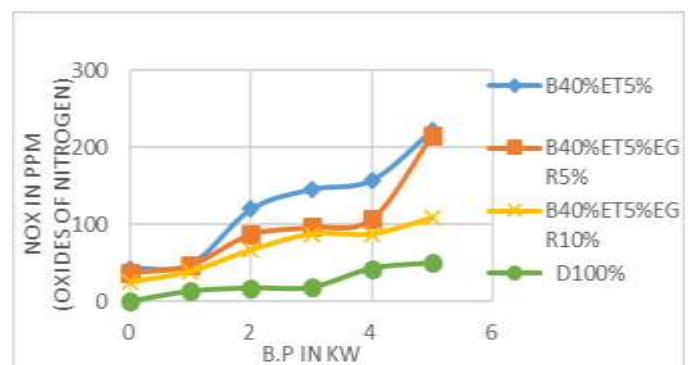
Fig -15: Variation emission of oxides of nitrogen with brake power for blend B40% with ethanol 5% without EGR, with EGR 5% and 10% .
