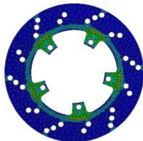
Fig.3 Analysis of Disc on Ansys
