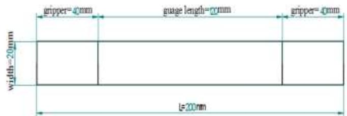
Fig 2. Standard tensile test specimen dimensions
