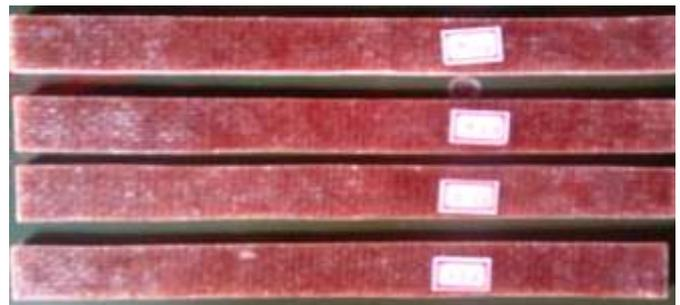
Fig 2. Tensile test specimens before test
