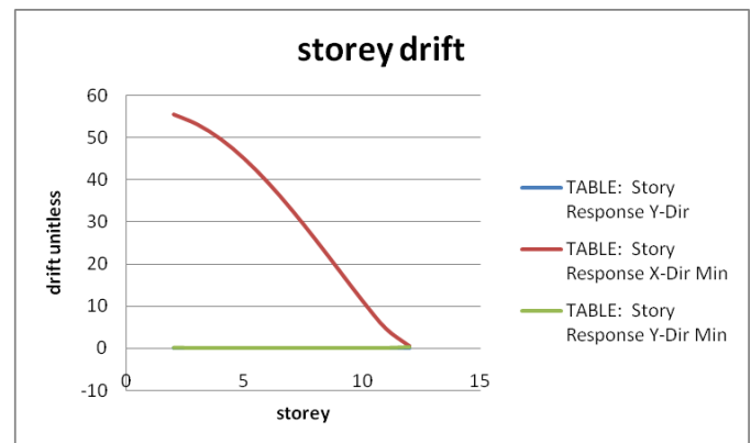
Fig 8 storey drift of double cross braced building
