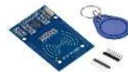
Radio-frequency identification uses electromagnetic fields to automatically identify and track tags attached to objects. The tags contain electronically stored information. Passive tags collect energy from a nearby RFID reader's interrogating radio waves. Active tags have a local power source and may operate hundreds of meters from the RFID reader.
