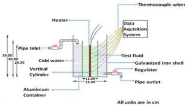
Fig.1: Experimental setup (17)
