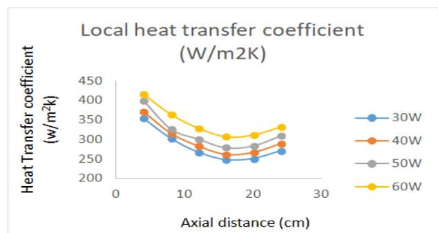
**Chart-6:** Variation of heat transfer coefficient with axial distance various heat input with vibration effect
