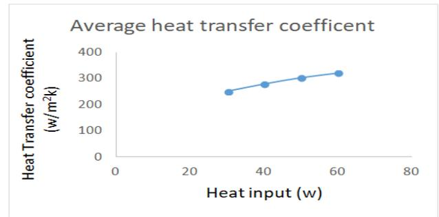
**Chart-4:** Variation of heat transfer coefficient with heat input
