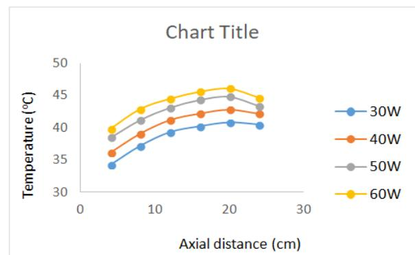
Chart-1: Surface temperature of the vertical cylinder along axial distance for without vibrations in the base fluid.
