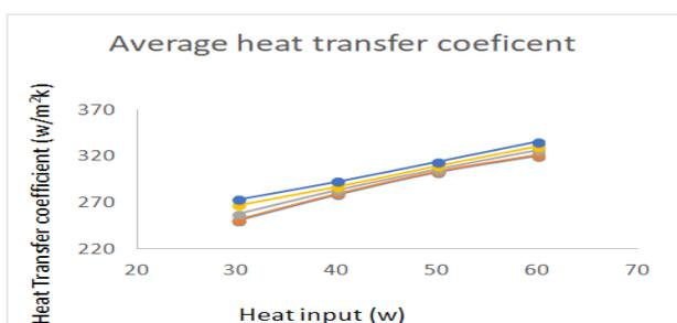
**Chart-9:** Variation of Average heat transfer coefficient with heat input
