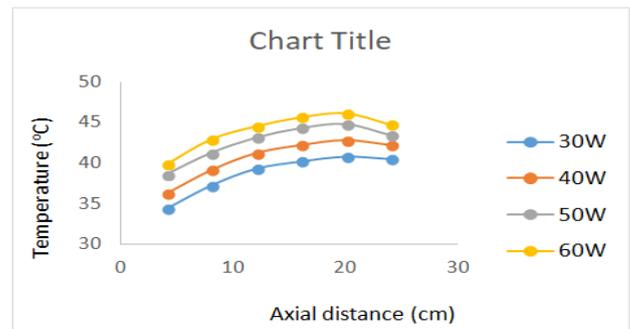
**Chart-5:** Surface temperature of the vertical cylinder along axial distance for with vibrations in the base fluid.
