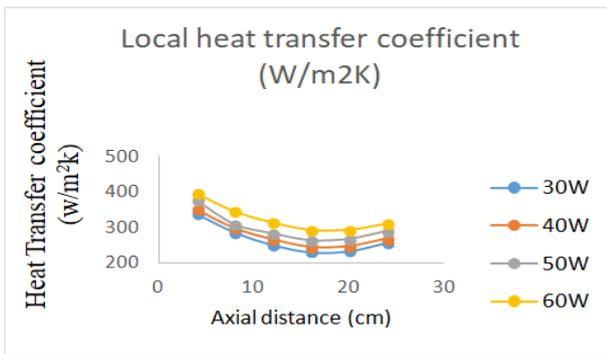
**Chart -2:** Variation of heat transfer coefficient with axial distance various heat input
