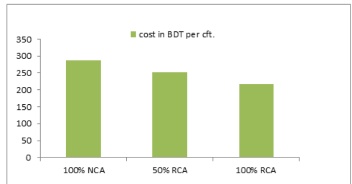
Figure-7: Cost in BDT per cft concrete of 100% NCA, 50% RCA and 100% RCA
