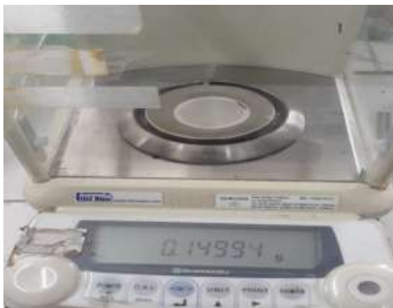
Fig. 7: Weight monitoring of filter paper for PM 2.5 concentration
