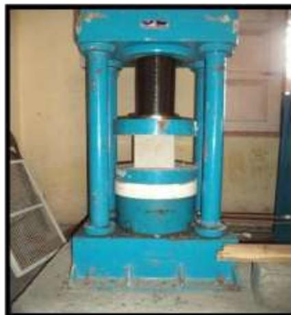
Fig 2 Compressive strength test set up
