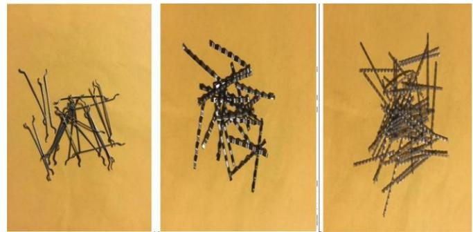
Hooked end steel      Crimped steel      Crimped PPI
