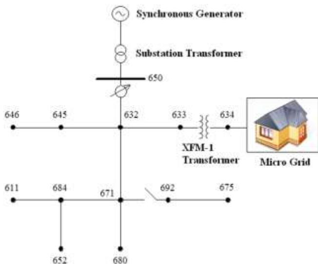
**Fig -4:** IEEE 13 buses modified system
