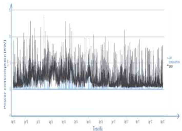
**Fig -6:** Total consumption graphs for 10 houses for a year. (Power Consumption(kW)-Time(h))
