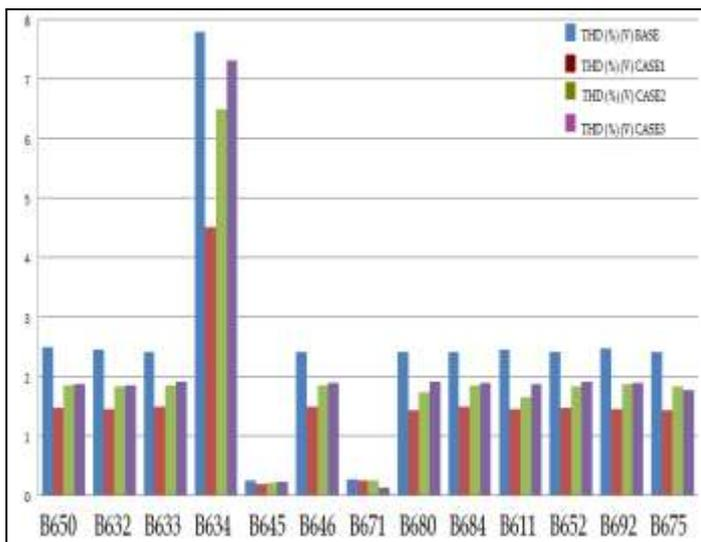
**Fig -9:** Voltage (THD) (%) of the 13-bus system for different situations
