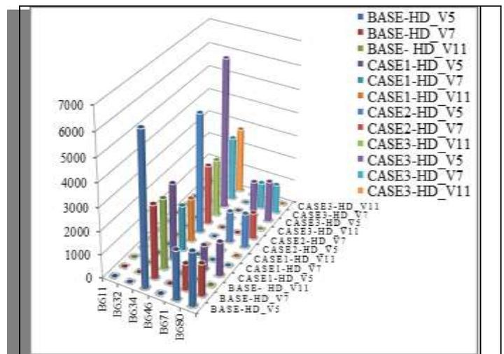
**Fig -10:** Voltage (THD) (%) of the 13 bus system for different situations
