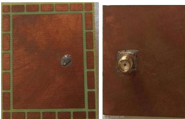
Fig 4(c) & 4 (d): Fabricated antennas with top view and bottom view of Patch with EBG
