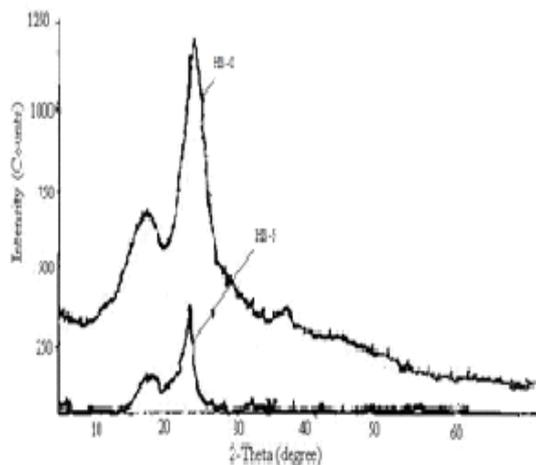
Fig -2: XRD patterns of untreated and pretreated sawdust samples from hardwood for hydrothermal treatment
