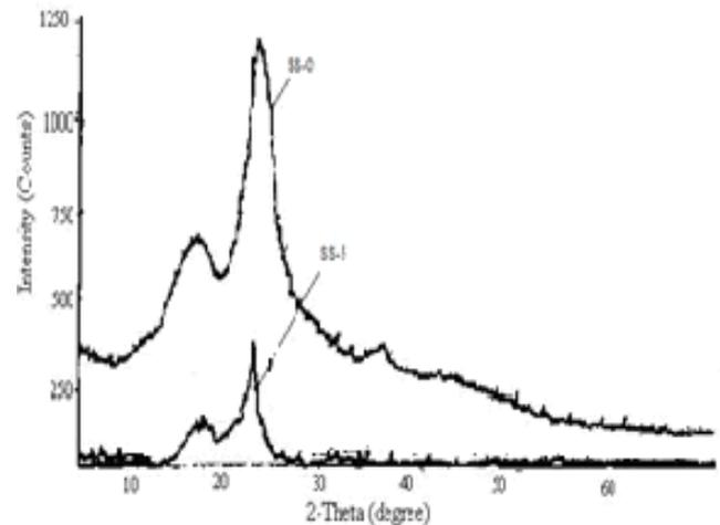
Fig -3: XRD patterns of untreated and pretreated sawdust samples from softwood for hydrothermal treatment
