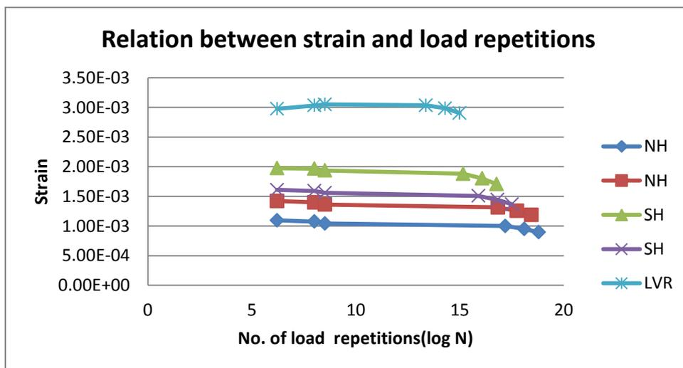
Chart-1 Permanent Deformation versus Load cycles
