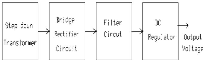
Fig- 2.1: Block diagram for power supply
