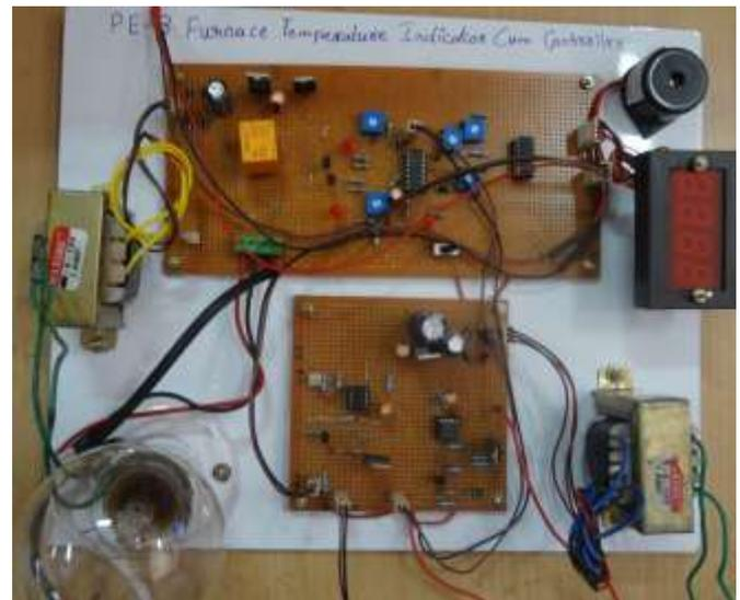
Fig- 6.1: Basic Indicator cum controller kit
