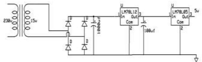
Fig- 4.1: Circuit diagram for Power Supply
