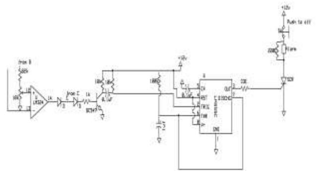
Fig- 5.3: Circuit diagram for Testing lower Temperature Alarm Point
