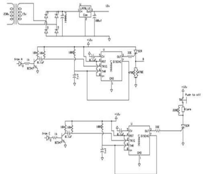
Fig- 3.2: Circuit diagram for Regulators
