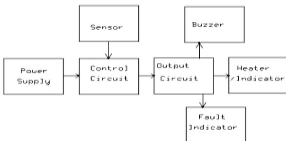
Fig-2.2:Block diagram for Main panel
