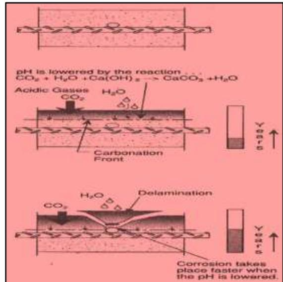
Fig.6 process of carbonation of concrete
