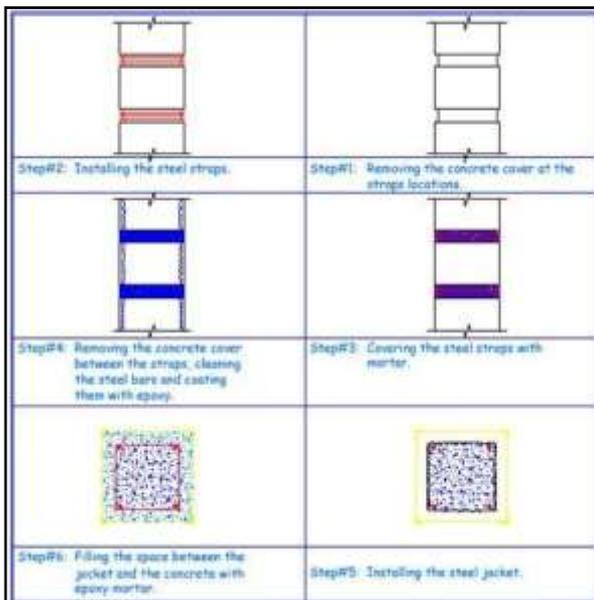
Fig.9 Steel Jacketing of a Column
