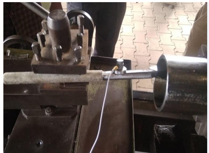
Figure 10: Sensor mounted on tool with glass fiber lamination
