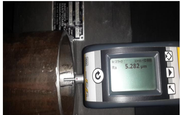
Figure 12: Surface roughness test machine
