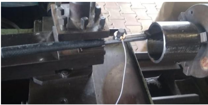
Figure 11: Sensor mounted on a tool with carbon fiber lamination
