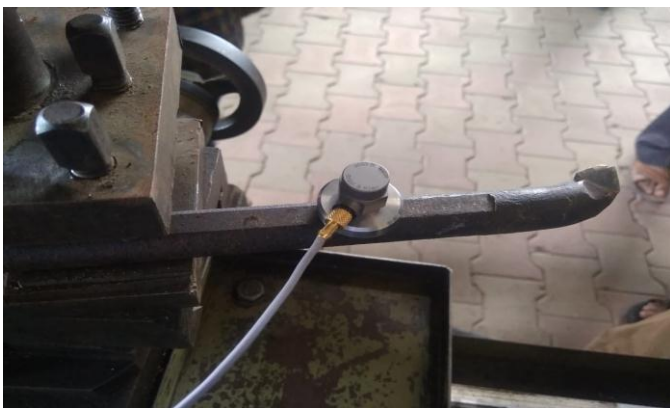
Figure 9: Sensor mounted on tool without lamination
